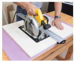
Using the GCX Clamp as your guide, plug in and power on the saw, then make the cut.
