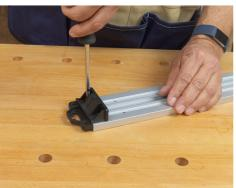
Using a phillips head screwdriver, remove the Fixed Jaw on one of the clamps.
