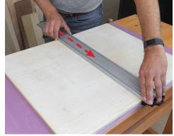
Align the clamp edge to the offset marks on your board and push the Sliding Cam Lock against the edge of your stock.
