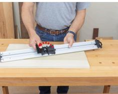
Open the Sliding Cam Lock 3 to the unlocked a position
