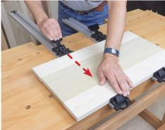
While holding the fixed jaw, slide the Sliding Cam Lock Jaw 3 firmly against the other side of your stock.
