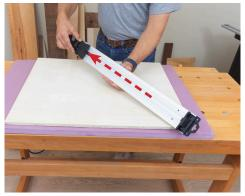
Slide the Sliding Cam Lock Jaw far enough away from the fixed end to fit your board in between the jaws.
