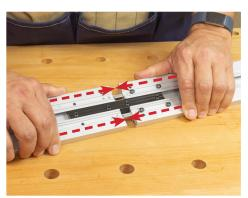
Align and insert the bars into the other aluminum body. Align the holes accordingly.
