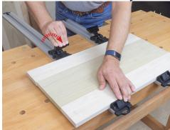
While holding the clamp down, secure stock by locking Sliding Cam Lock. Allow to dry.
