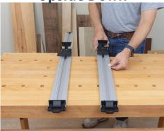
Flip the two clamps upside down parallel to each other as shown here. Place your glued up stock in between the jaws.
