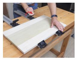
While holding the clamp down, secure stock by locking Sliding Cam Lock
