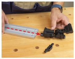
Slide the Sliding Cam Lock 3 assembly out through the open end of the second clamp 2.
