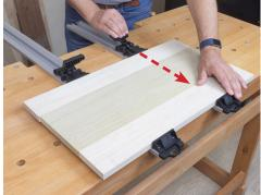
While holding the fixed jaw, slide the Sliding Cam Lock Jaw 3 firmly against the other side of your stock.
